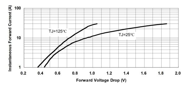
Fig.3-Typical Forward Voltage Drop Characteristics
